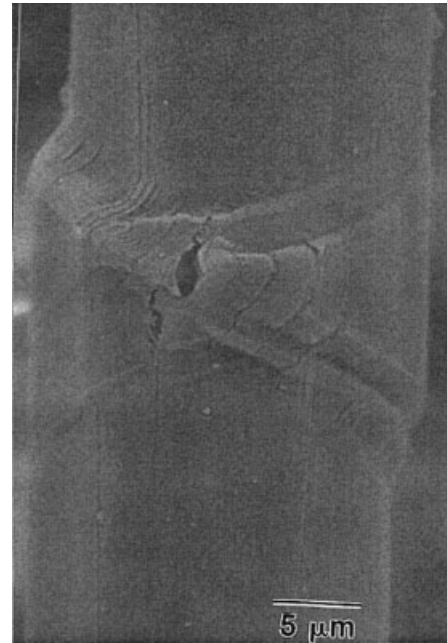
Figure 17 Kink band in experimental PBO fiber.
